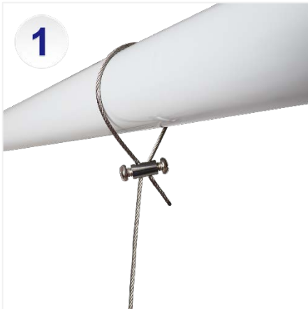
1. The wire rope passes through the beam and is fixed by the Double hole wire rope lock (Cable Looping Gripper)
